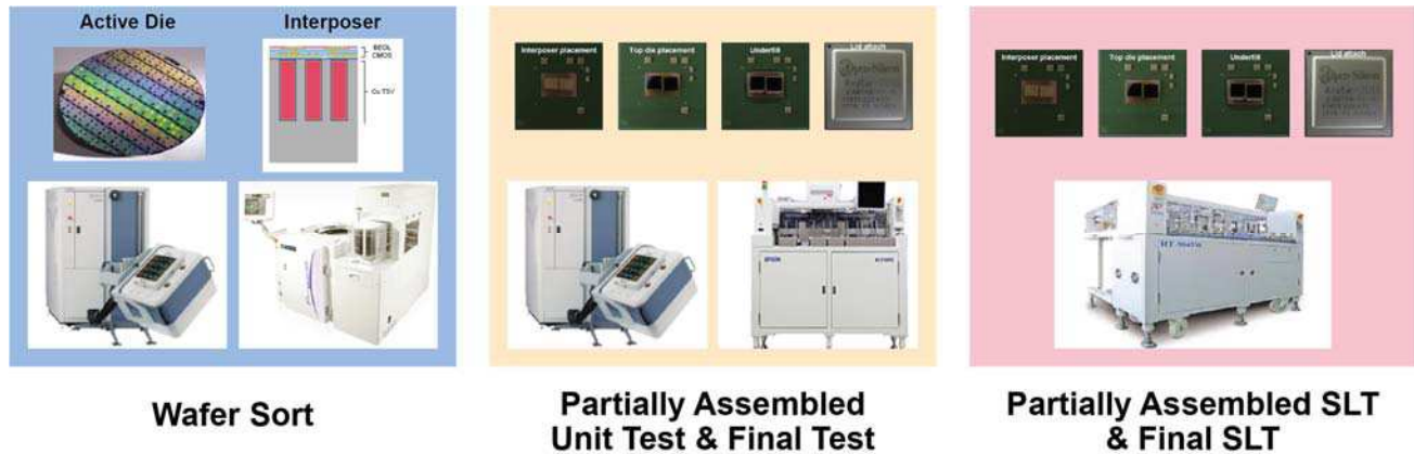
Figure 4: Test Insert Points for Advanced Packages
