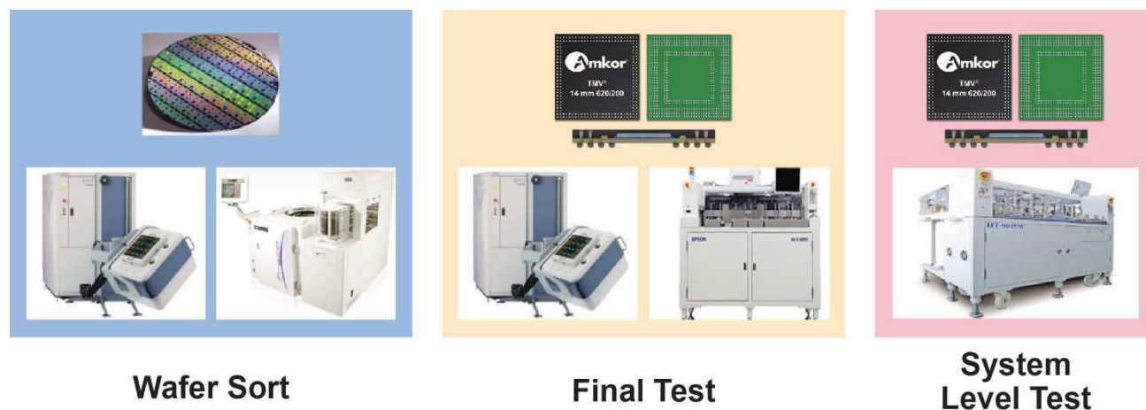
Figure 1: Traditional Test Insertion Points for Semiconductor Test
